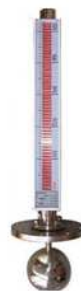
Model No. : 09 - RI TOP - MOUNTED MAGNETIC LEVEL INDICATOR TYPE : MAGNETIC MOUNTING : TOP GUIDE PIPE : A PERFORATED G.I/SS.304/316/PP ETC. PIPE FLANGE : 4" /6"NB, ASA 150 C.S./ANY MOC FLANGE TEST PRESSURE : 5 KG/CM-2 / HIGH PRESSURE AS PER REQUEST
